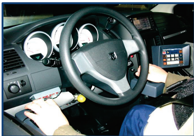
Electronic Gas/Brake Lever used with left arm and Electronic Wheel used with right arm for steering.
